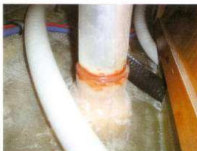
Aluminium extension tube is laminated into the hull with an epoxy seal
